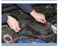
The most basic voltage drop check is between the negative battery post and the engine. Check this voltage under load, such as when starting. It should be less than half a volt, even when cranking.
