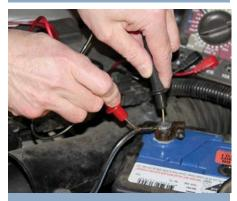
If you are still chasing the source of the voltage drop between the battery and the engine or chassis, then check the drop between the conductor and the battery post
